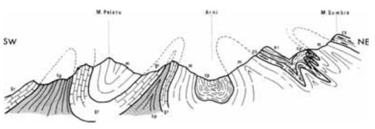
Figure 20 - The structure of the Arni valley after Lotti (1881a, b). sp: Paleozoic phyllites, gr: Triassic dolomites, m: marbles, cs: certy limestones, cp: calcschists, ar: metasandstones flysch.
