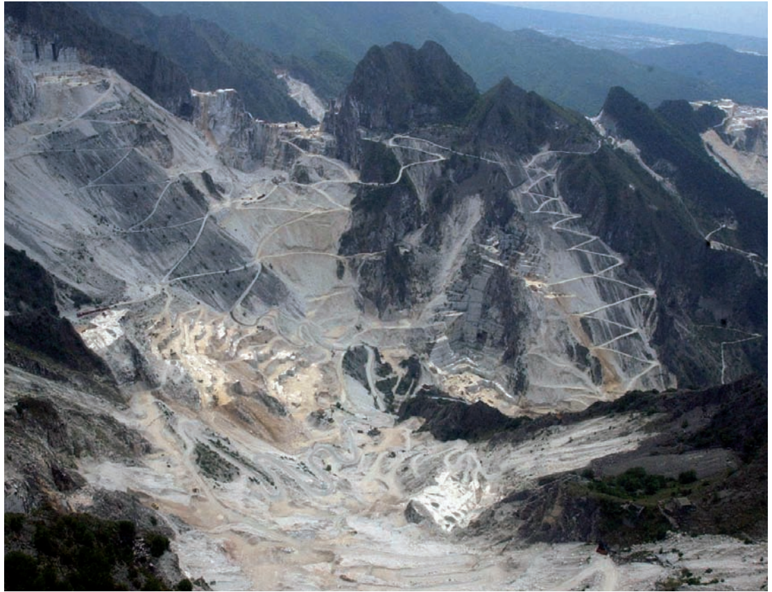
FIG. 18 - Overview of Ravaccione area in the Torano basin, Carrara: active (light grey) and ancient (dark grey) quarries and quarry dump deposits (ravaneti, photo C. Baroni).
